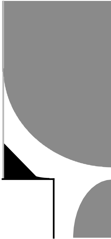
Figure 6.3. Cell flow for high Bingham number. The shaded regions are where the fluid is plastic, but moving. The dead zone is in black.
