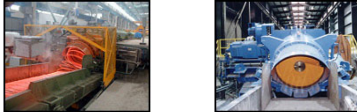
Figure 1: The Morgan Construction laying head. The photo on the left shows the laying head in action with hot coils of steel exiting the machine. The photo on the right shows a close up view of the laying head. Photos courtesy of Morgan Construction.
